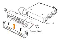
The remote head cable uses an 8 pin telephone style connector. Plug the cable from the remote head into the socket in the FRONT of the MAIN unit. Plug the MICROPHONE (6 pin plug) into the front of the REMOTE HEAD unit. (Alternatively the microphone can be plugged into the rear microphone socket on the main unit.
